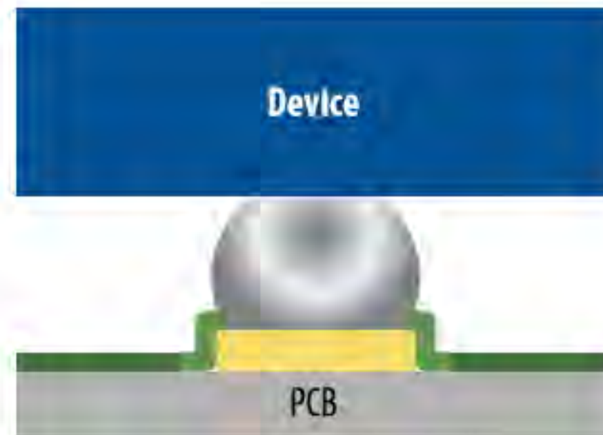
Symmetrical solder ball (Regardless of registration) Solder mask defined
